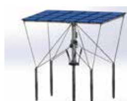
Screw Pile 螺旋樁
